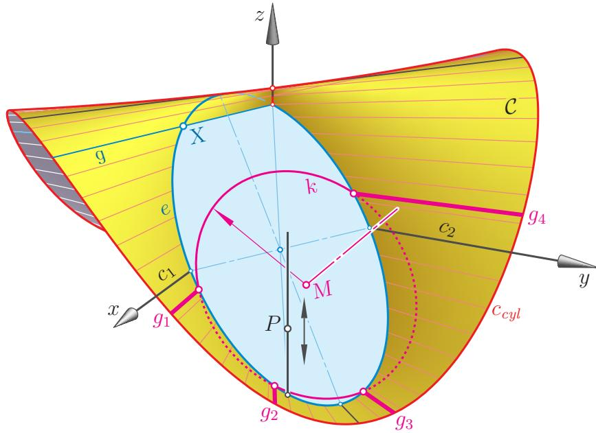
Fig. 9. The ellipse  $e$  is the pedal curve of  $\mathcal{C}$  w.r.t. the point  $P$ . There are infinitely many spheres contacting the four concyclic generators  $g_1, \dots, g_4$  of  $\mathcal{C}$ . The center of a contacting sphere must be located on the vertical line through  $P$  and on the axis of the circle  $k$ .
