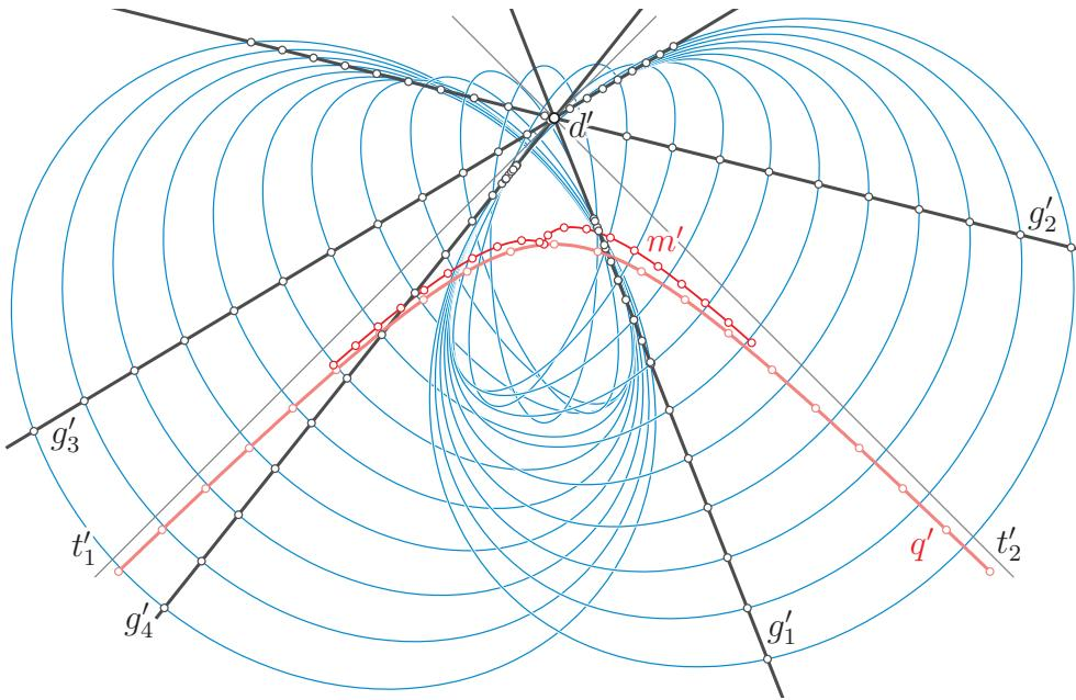
Fig. 12. Top view of a sample of circles of the canal surface through the four concyclic lines  $g_1, \dots, g_4$  on the Plücker conoid with torsal generators  $t_1, t_2$  and double line  $d$ . The hyperbola  $q'$  is the top view of the spine curve and  $m'$  that of the curve of circle centers.
