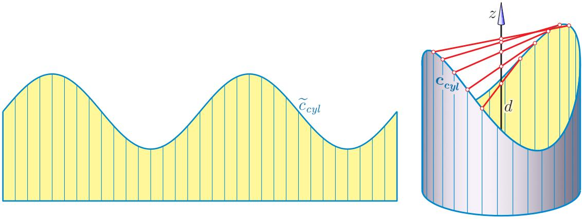
Fig. 2. The intersection  $c_{cyl}$  of Plücker's conoid  $\mathcal{C}$  with a right cylinder about the double line  $d = z$ -axis appears in the cylinder's development as two periods of a Sine curve. The generators of  $\mathcal{C}$  connect opposite points of  $c_{cyl}$ .
