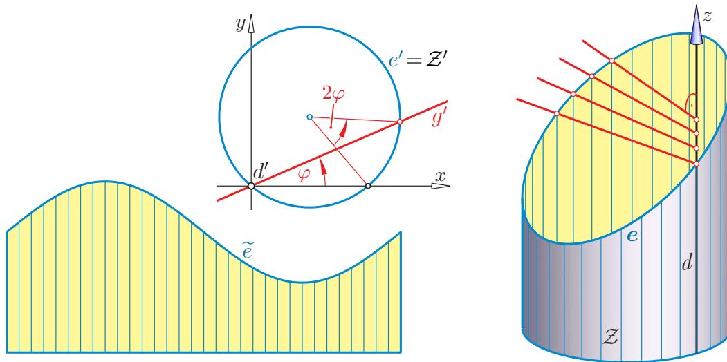
Fig. 3. The intersection  $e$  of the conoid  $\mathcal{C}$  with a right cylinder  $\mathcal{Z}$  through the double line  $d$  appears in the cylinder's development as one period  $\tilde{e}$  of a Sine curve. The generators of  $\mathcal{C}$  meet  $e$  and intersect  $d$  orthogonally.
