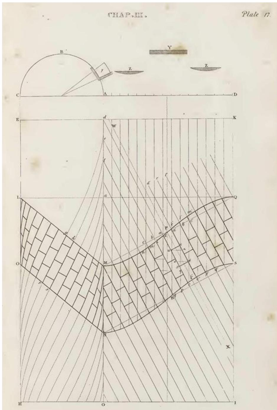
Obr.15. Nicholson A Practical Treatise on the Art of Masonry and Stone-cutting
