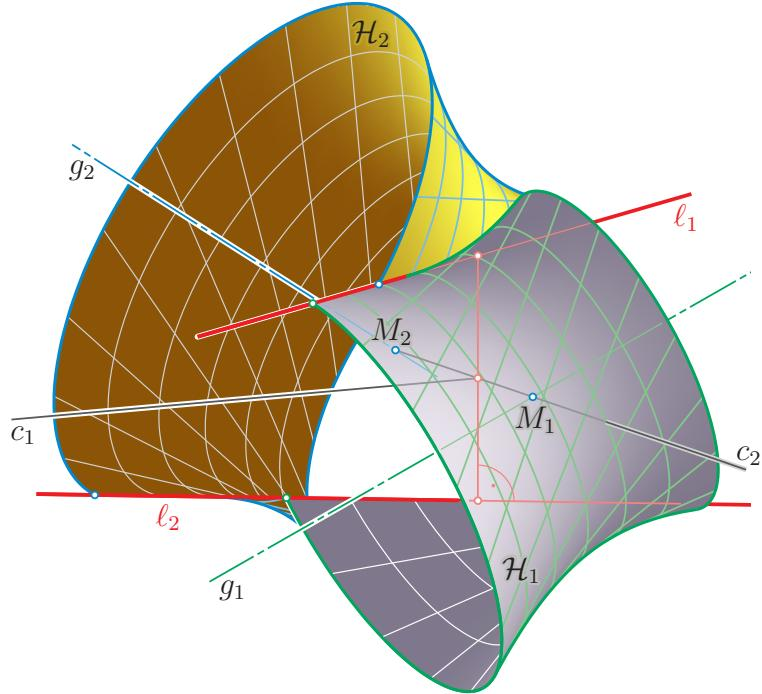
Fig. 6. Two hyperboloids of revolution  $\mathcal{H}_1, \mathcal{H}_2$  through two skew lines  $\ell_1$  and  $\ell_2$ . The two hyperboloids with respective centers  $M_1, M_2$  and axes  $g_1, g_2$  on the bisecting paraboloid (with vertex generators  $c_1, c_2$ ) share the secondary semiaxis.
