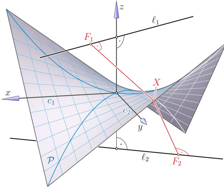
Fig. 5. The bisector of two skew lines  $\ell_1$  and  $\ell_2$  is an orthogonal hyperbolic paraboloid  $\mathcal{P}$  which contains the axes of symmetry  $c_1, c_2$  of  $\ell_1$  and  $\ell_2$  as vertex generators.
