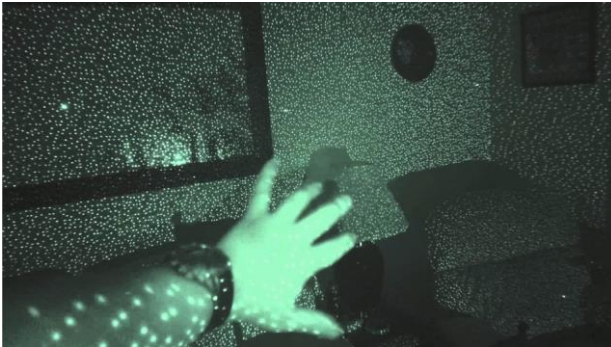
Fig. 2: Laser mesh projected by Kinect into the space
