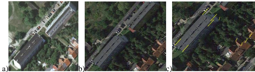
Fig. 7 Images of two identical adjacent buildings featured in Google maps at different times a) earlier b) current c) projections constructed on the basis of images (yellow sections)
